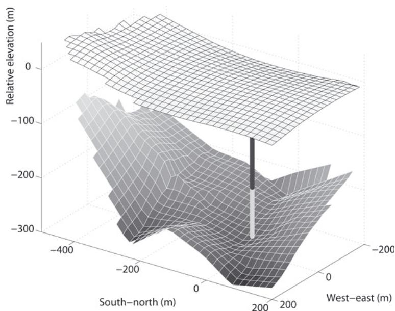
**Fig. 5.** Oblique view of the study site. Upper and lower surfaces show the glacier surface and bed, respectively. The grid size of the mesh is  $20 \text{ m} \times 20 \text{ m}$ . The vertical column indicates the drilling site, with dark gray representing the retrieved 180.17 m long ice core.
