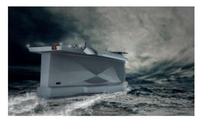
Inspired by airfoil techniques harnessed by the aviation and sailboat industries, *Vindskip*'s wind-powered propulsion enables a 63% reduction in CO<sub>2</sub>
