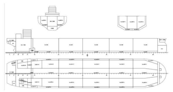
Figure 4: Minimal Ballast Water Ship VLCC design developed by Namura Shipbuilding Co., Ltd. in cooperation with the Shipbuilding Research Centre of Japan
