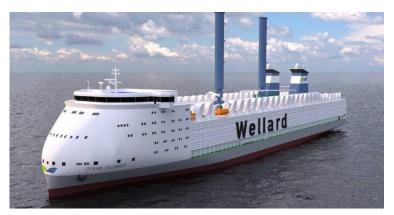
Figure 5: Flettner rotors fitted on a ship's weather deck (source: International Windship Association)
