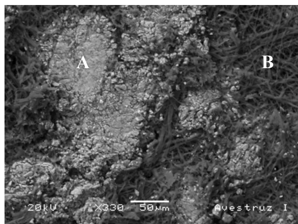
Figure 6: LVSEM image ostrich eggshell (inner side) in which calcite crystallites ( \text{CaCO}_3 ) are mineralized in a biopolymer.
