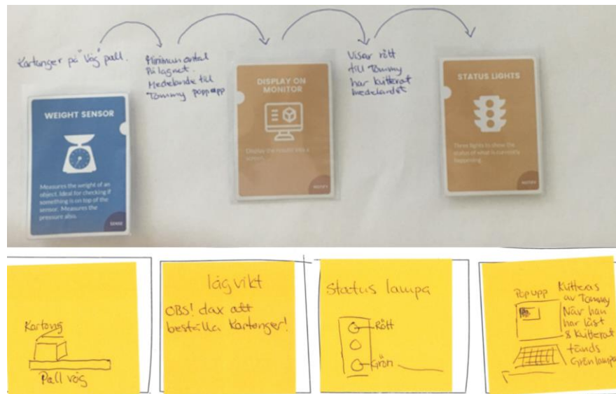
Figure 4. Above, conceptual solution: a weight sensor detects that more boxes are needed and notifies operators through a display and status lights. below, storyboard.
