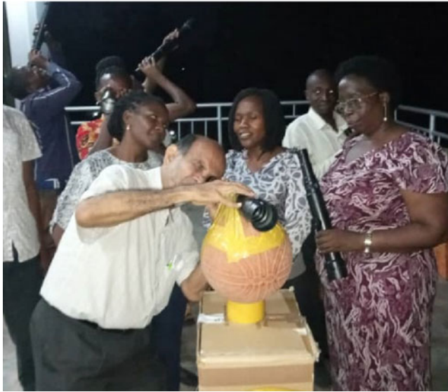
Figure 1. Need to innovate: Instead of a tripod, the telescope is taped to a football swiveled on a short cylinder
