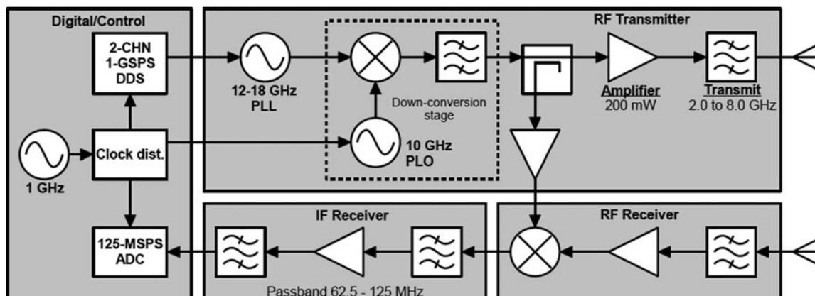
**Fig. 3.** Block diagram of the Snow Radar.
