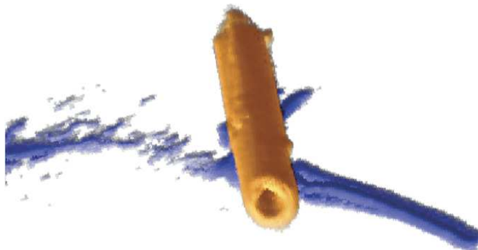
Figure 1: A three-dimensional DART [4] tomographic reconstruction rendering of an inorganic nanotube (orange) and the underlying amorphous carbon support (blue). The tilt series containing 3 487 images was recorded in only 3.5 s, limited by the rotation speed of the goniometer. Picture taken from [2].
