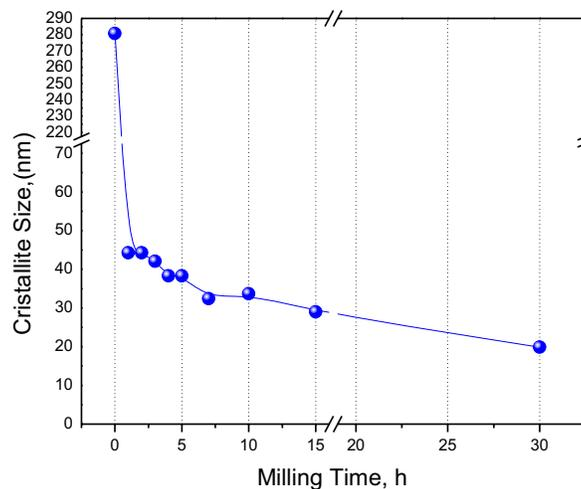
**Figure 1.** Graph showing crystallite size (CS) for Al<sub>2024</sub>/SiC nanocomposites containing 2.0, wt.% SiC milled for 0, 1, 2, 3, 4, 5, 7, 10, 15, 30 h.
