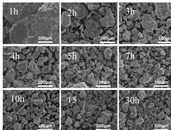
**Figure 2.** SEM micrographs of Al<sub>2024</sub>/SiC<sub>NP</sub> particle size milled for 1, 2, 3, 4, 5, 7, 10, 15 and 30h. shows the variation of size as a function of milling time.
