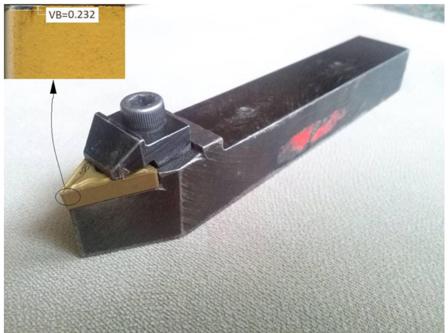
Fig. 4. Tool holder, tool insert type TNMG220408, and measured tool flank wear.
