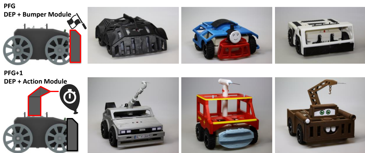
Figure 6. Physical products for the DEP with the bumper module and with the action module
