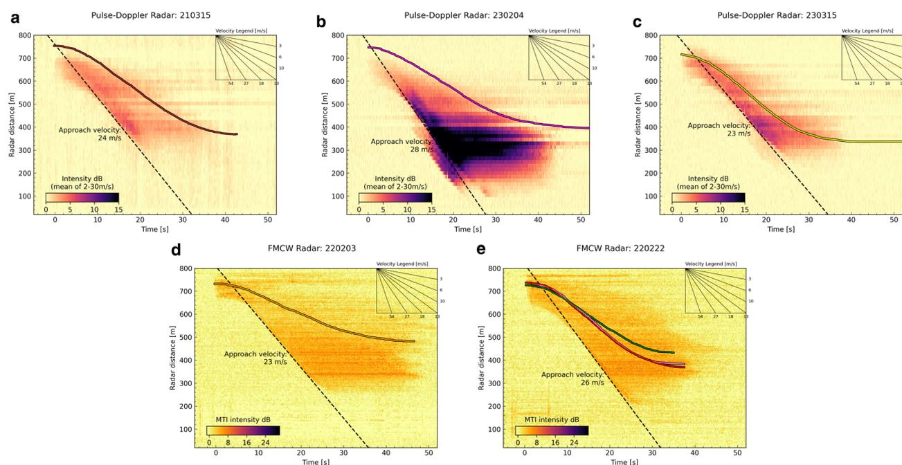
**Figure 7.** Range-time radar images show the avalanche motion and locate the AvaNode position in relation to the avalanche front. a, b and c are pulse-Doppler radar data, d and e are mGEODAR radar (FMCW-type) data. The maximum avalanche front velocity is indicated with a dashed black line and its angle corresponds to the apparent approach velocity in direction of the radar. AvaNodes with higher density are seen in panel B (magenta) and panel E (green).
