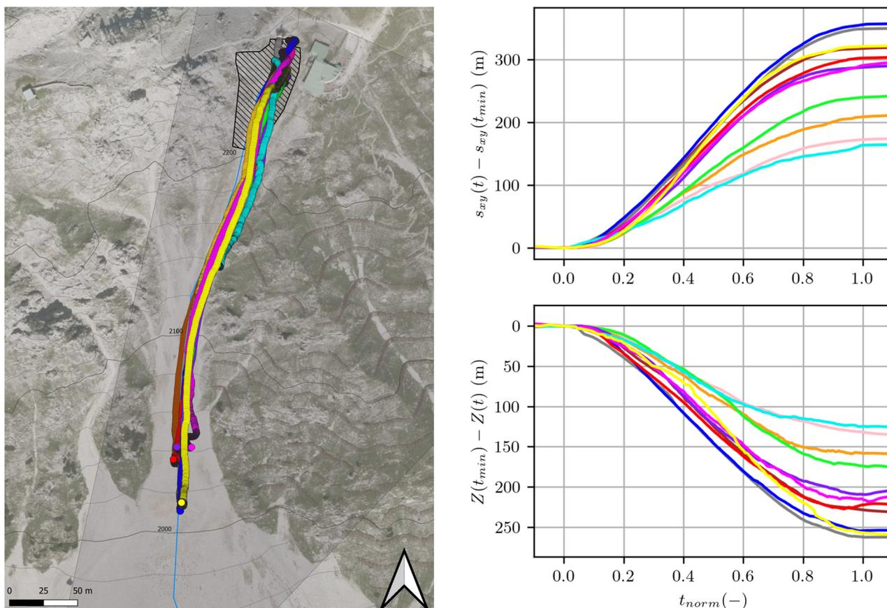
**Figure 4.** In the left panel, trajectories or GNSS positions of all avalanche experiments are displayed. The spacing of the isochronous sampled position data indicates the flow velocity, e.g. the herein called position velocity  $v_p$ . The dot size is set to 5 m, which corresponds to the accuracy stated by the manufacturer. The hatched area represents the release zone. In the right panel the projected travel length  $\Delta s_{xy}(t)$  and the altitude difference  $\Delta Z(t)$  are shown.
