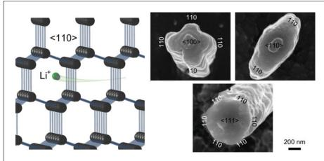
Upon lithiation, the initially circular cross sections of crystalline Si nanopillars with <100>, <110>, and <111> axial orientations expand into cross, ellipse, and hexagonal shapes, respectively. A high-speed lithium ion diffusion channel along the <110> direction causes preferential volume expansion along this direction. Reproduced with permission from *Nano Lett*. (DOI: 10.1021/ nl201787r). © 2011 American Chemical Society.
