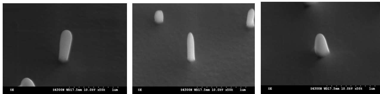
FIG. 2. Types of the deposits. (a) Deposit of Type I grown at 20 keV, 36 pA and -28°C, (b) Deposit of Type II grown at 20 keV, 383 pA and 0°C, (c) Deposit of Type III grown at 20 keV, 1420 pA and 15°C.
