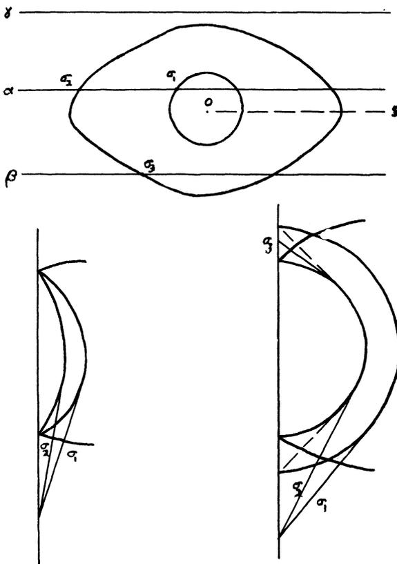
Fig. 13. Formation after reflection of supersonic boundary wave sheets. (a) early stage, (b) late stage. Above: normal surface and boundary cylinder.
