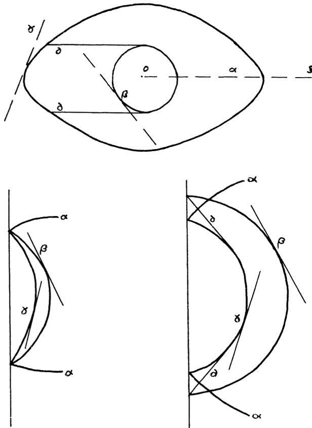
Fig. 12. Reflection of a slow incident wave front. (a) early stage, (b) late stage. Above: normal surface.
