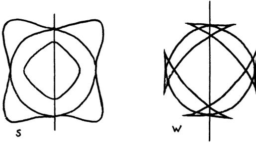
Fig. 7. Inverse and wave surfaces of nickel in cross-section. Cubic symmetry.
