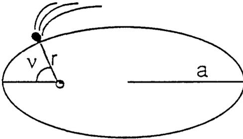
Figure 1. The cometary ellipse showing the true anomaly ( $\nu$ ).
