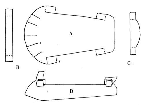
Fig. 3. A. Zinc sheet cut for folding into arm shield. Dotted lines indicate tags bent back. *t*, tag; *s*, slits to enable shield to be moulded to elbow. B. Zinc strip with ends folded to form band below elbow. C. The same at wrist. D. Shield assembled on arm.
