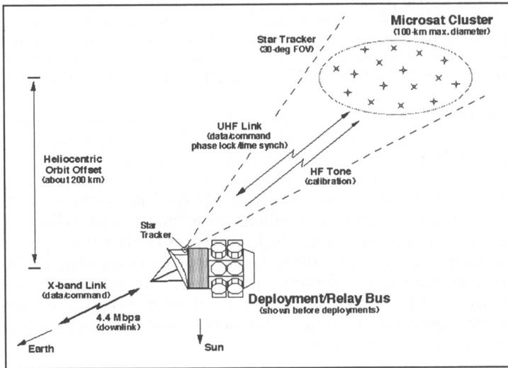
Figure 1. Basic design of the ALFA mission after deployment.
