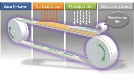
Figure 1. Schematic of process developed at Brown University to form large-area single-crystal substrates using electrochemical deposition and etching.
