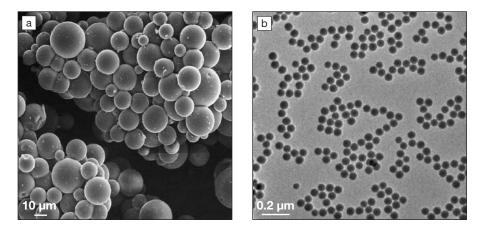
Figure 1. (a) Microparticles (scale bar: 10 µm) and (b) nanoparticles (scale bar: 200 nm) demonstrating the size ranges that can be obtained using CeramiSphere technology.
