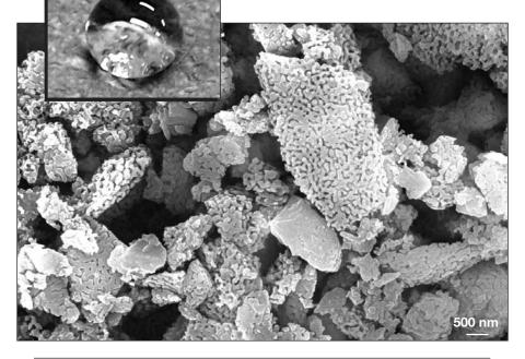
Figure 1. Scanning electron micrograph of nanotextured glass powder grains. The inset shows a water drop on a piece of fabric.
