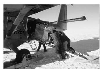
**Fig. 6.** Unloading the winch frame from the Twin Otter using H-section ramps.
