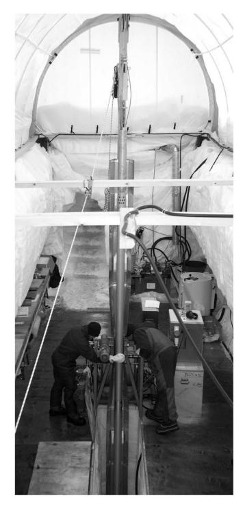
Fig. 9. The covered drilling pit, with deep ice-core drill system.
