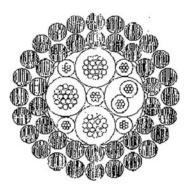
Fig. 8. Cross-section of the drill cable.
