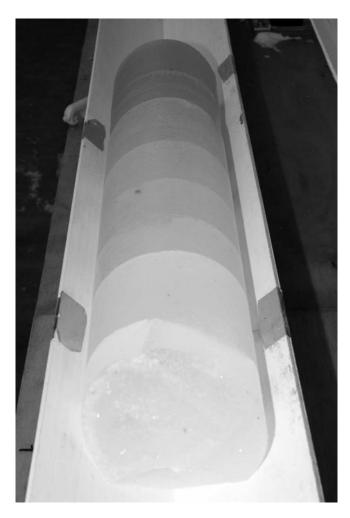
**Fig. 13.** The final 0.5 m of ice core before the basal sediment was encountered; the deepest ice is furthest from the camera. The banding is due to horizontal cracks in the core from the drilling which were not apparent on earlier cores. Below this section, no further ice was recovered, with only fine sand sediment recovered from subsequent drilling runs. Note the occasional larger conglomerate particles in the ice.
