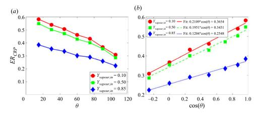
Figure 16. (a) Dependence of average evaporation rate in CRP ( $ER_{CRP}$ ) on contact angle ( $\theta$ ). (b) Dependence of  $ER_{CRP}$  on  $\cos(\theta)$ .
