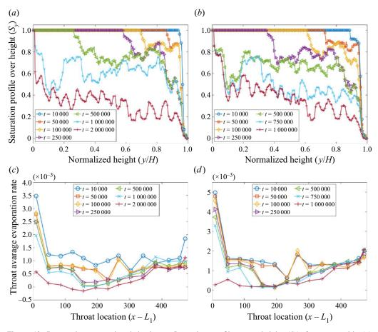
Figure 10. Pore-scale evaporation behaviours. Saturation profiles over height  $(S_y)$  for cases with (a)  $Y_{vapour,in} = 0.9$  and (b)  $Y_{vapour,in} = 0.1$ . Pore-local evaporation rates at the top surface of the porous medium (y = H) for (c)  $Y_{vapour,in} = 0.9$  and (d)  $Y_{vapour,in} = 0.1$ .
