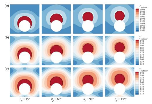
Figure 4. Validation of contact angle implementation scheme at different prescribed contact angles:  $\theta_p = 15^\circ$ ,  $\theta_p = 60^\circ$ ,  $\theta_p = 90^\circ$  and  $\theta_p = 135^\circ$ . Three initial water vapour mass fractions in the gas phase are considered: (a)  $Y_{vapour,i} = 0.95$ , (b)  $Y_{vapour,i} = 0.5$  and (c)  $Y_{vapour,i} = 0.1$ .
