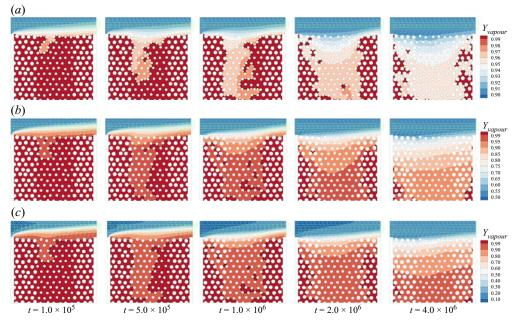
Figure 9. Time evolution of liquid distribution in the porous medium for cases with  $\theta = 15^{\circ}$ . The arrows show the velocity field, the solid black lines indicate the liquid–gas interface locations and the contours present the vapour mass fraction: (a)  $Y_{vapour,in} = 0.9$  (supplementary movie 1), (b)  $Y_{vapour,in} = 0.5$  (supplementary movie 2) and (c)  $Y_{vapour,in} = 0.1$  (supplementary movie 3).
