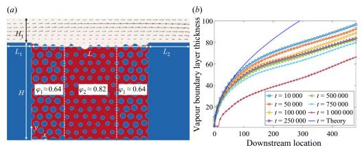
Figure 8. (a) Simulation set-up. A dual-porosity medium filled with liquid water is installed in the middle bottom. A mixture gas (dry air + water vapour) is convectively blown in the top channel, with a Poiseuille inflow velocity profile. (b) Development of vapour boundary layer thickness for a typical case. The solid line is the Blasius solution.
