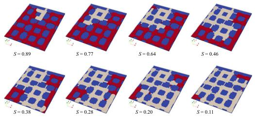
Figure 20. Evolution of the liquid distribution in the network at different liquid saturations S.
