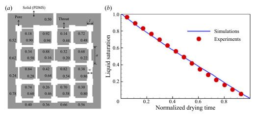
Figure 6. Validation with microfluidic evaporation experiment. (*a*) Structure of the network taken from Wu *et al.* (2016), copyright Elsevier (PDMS, polydimethylsiloxane). (*b*) Variation of the liquid saturation with drying time normalized by the total drying time.
