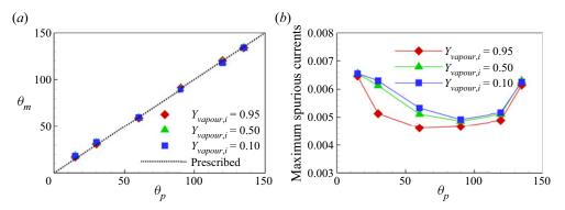
Figure 5. (a) Measured contact angles  $\theta_m$  versus prescribed contact angle  $\theta_p$ . (b) Comparison of the maximum spurious currents for different cases.
