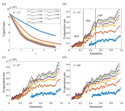
Figure 11. Global evaporation behaviours. (a) Time evolution of the residual liquid mass for cases with  $\theta = 15^{\circ}$ . Evaporation curves (evaporation rate versus mean liquid saturation) for cases with  $\theta = (b) 15^{\circ}$ , (c)  $45^{\circ}$  and (d)  $60^{\circ}$ .
