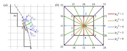
Figure 1. (a) Sketch of the geometric function scheme to achieve a prescribed contact angle  $\theta_p$  at the solid point S on a curved surface. (b) The D2Q25 lattice is used to calculate the unit normal vector  $\mathbf{n}_s$  in (a).
