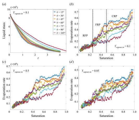
Figure 15. Global evaporation behaviour. (a) Time evolution of the residual liquid mass for cases with  $Y_{vapour,in} = 0.1$  and different contact angles  $\theta$ . Evaporation curves for cases with  $Y_{vapour,in} = (b) 0.1$ , (c) 0.5 and (d) 0.85.
