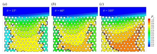
Figure 17. Normalized vapour pressure distribution with  $Y_{vapour,in} = 0.5$  at S = 0.2 for different contact angles: (a)  $\theta = 15^{\circ}$ , (b)  $\theta = 60^{\circ}$  and (c)  $\theta = 105^{\circ}$ .
