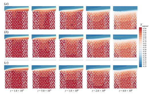
Figure 14. Time evolution of the liquid distribution in the porous medium for cases with  $Y_{vapour,in} = 0.1$ . The arrows show the velocity field, the solid black lines indicate the liquid–gas interface locations and the contours are for the vapour mass fraction distributions. Contact angle (a)  $\theta = 30^{\circ}$  (supplementary movie 4), (b)  $\theta = 60^{\circ}$  (supplementary movie 5) and (c)  $\theta = 105^{\circ}$  (supplementary movie 6).
