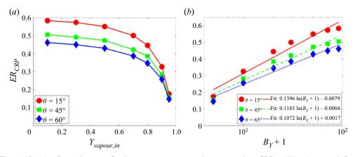
Figure 12. (a) Dependence of the average evaporation rate in CRP  $(ER_{CRP})$  on inflow vapour concentration  $(Y_{vapour,in})$ . (b) Dependence of  $ER_{CRP}$  on the mass transfer number  $B_Y = (Y_{vapour,1} - Y_{vapour,in})/(1 - Y_{vapour,1})$ . The plot is on a semi-log scale.
