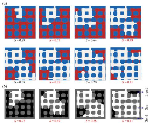
Figure 7. Evolution of the liquid distribution in the network at different liquid saturations *S*. (*a*) The LBM simulations in the present work. (*b*) Experimental images taken from Wu *et al.* (2016), copyright Elsevier.
