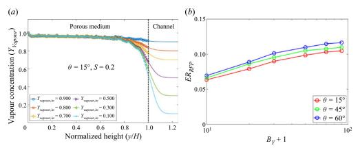
Figure 13. (a) Comparison of the vapour concentration profiles for different cases with  $\theta = 15^{\circ}$  at S = 0.2. (b) Dependence of the average evaporation rate in RFP (*ER<sub>RFP</sub>*) on the mass transfer number  $B_Y$  for different contact angles. The plot is on a semi-log scale.
