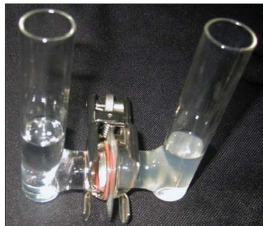
Figure 1. Method for producing chitosan nanoparticles by flow through a nanoporous membrane. (Images courtesy of Richard N. Zare, Chair, Department of Chemistry, Stanford University.)
