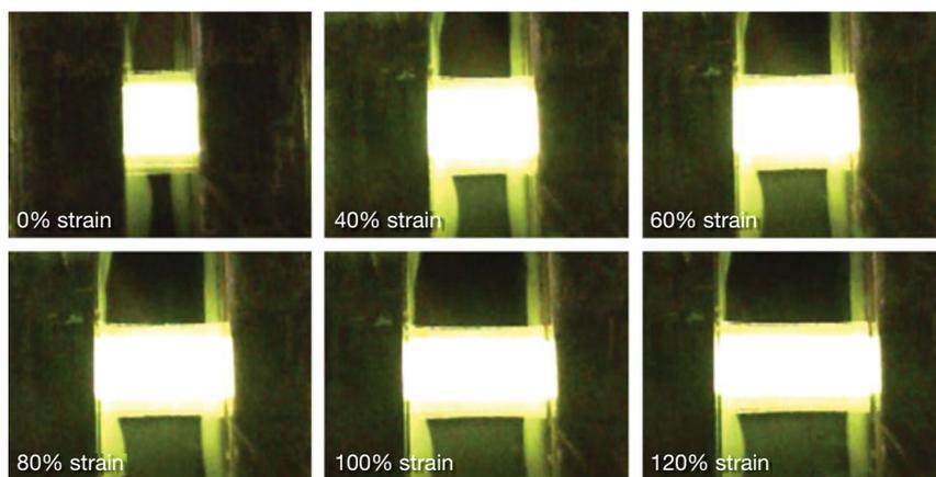
Device characterization of a stretchable polymer light-emitting electrochemical cell. Reproduced with permission from *Nat. Photonics*, **7** (2013), DOI: 10.1038/nphoton.2013.242; p. 817. © 2013 Macmillan Publishers Ltd.
