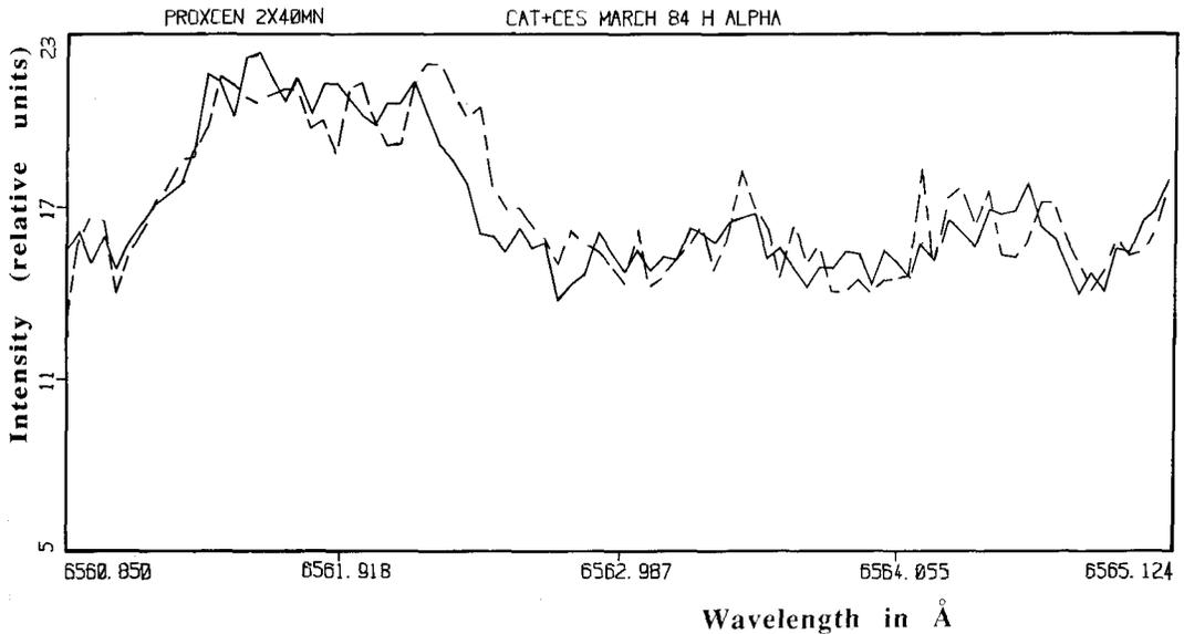
Fig. 5. Comparison between two 40 min exposure spectra of Prox Cen in H $\alpha$  observed with the CAT 1.4 m telescope + CES spectrometer and reticon at ESO. The superposition shows an asymmetric broadening of the line, possibly due to a Doppler-shifted component. Provided the S/N and time resolution are sufficient, line asymmetries and velocity components can be monitored as flare motion diagnostics, as suggested in these H $\alpha$  studies.
