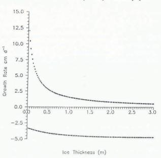
Fig. 1. Freezing rate in cm  $d^{-1}$  as a function of thickness in meters for winter (upper curve) and summer (lower curve).
