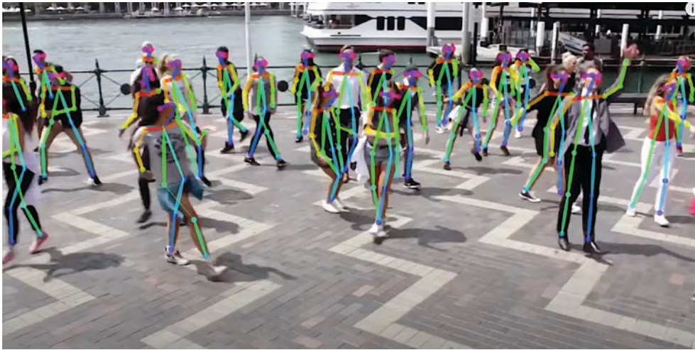
Figure 4. Software tracks dancers' movements in real-time by superimposing color-coded dots and lines on their bodies. "Realtime Multi-Person 2D Human Pose Estimation using Part Affinity Fields, CVPR 2017 Oral" posted by Zhe Cao, 6 December 2016, www.youtube.com/watch?v=pW6nZZeWlGM . (Screengrab by TDR)
