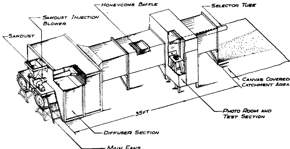
*Fig. 1. Schematic drawing of low-speed wind tunnel used to study model precipitation gages under simulated snow-storm conditions*
