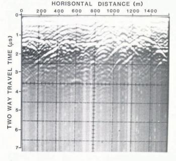
Fig.4. The bottom reflection is hidden by diffraction hyperbolae. Each hyperbola originates from one reflection point.
