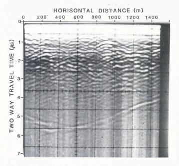
Fig.3. Bottom reflection of good continuity and sufficient amplitude.
