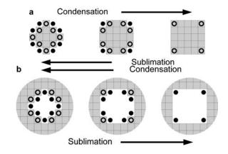
**Fig. 1.** Faceting model based on Kossel crystal explanation. Circles and dots correspond to preferential sublimation and condensation sites, respectively. (a) For convex shapes, condensation leads to faceting while sublimation generates a rounding of the grains. (b) For concave shapes, the reverse behaviour is observed.
