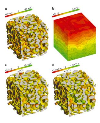
**Fig. 2.** Three-dimensional representations of a slightly faceted snow sample imaged after 3 weeks of TG metamorphism (TG = 3 K m<sup>-1</sup>). (a) Curvature map; (b) temperature field; and (c,d) computed incoming matter fluxes for the diffusive (c) and reactive (d) models. Edge size of the volume: 300 voxels  $\sim$ 3 mm.
