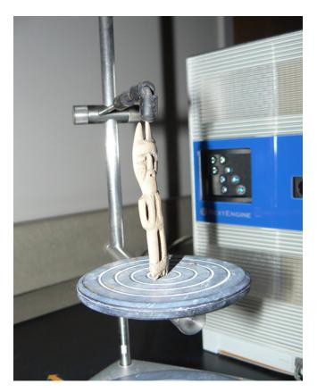
**FIGURE 1.** Using a NextEngine Desktop 3D Scanner to create a digital model of a Susquehannock bone comb fragment broken during manufacture that is in the collections of the State Museum of Pennsylvania, Harrisburg.
