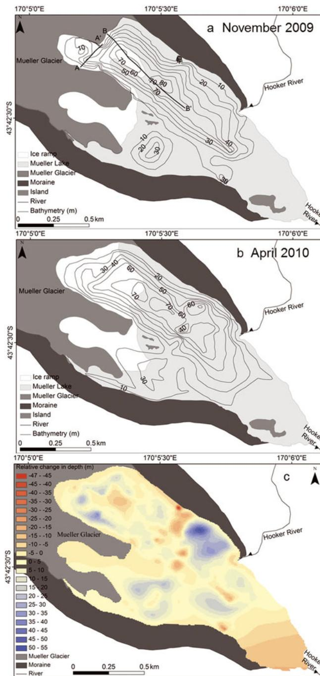
**Fig. 3.** Subaqueous terminal morphology and bathymetry of Mueller Lake: (a) November 2009, where lines A–A' and B–B' show the location of sub-bottom profile images in Figure 4; (b) April 2010; (c) the relative change in lake depth between (a) and (b). Negative values (red) show a decrease in depth, and positive values (blue) show an increase in depth.
