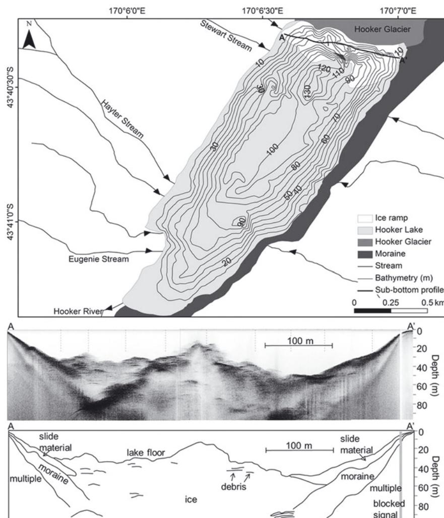
**Fig. 5.** Subaqueous terminus morphology and bathymetry of Hooker Lake in November 2009. Line A–A' shows the location of the sub-bottom profile image.
