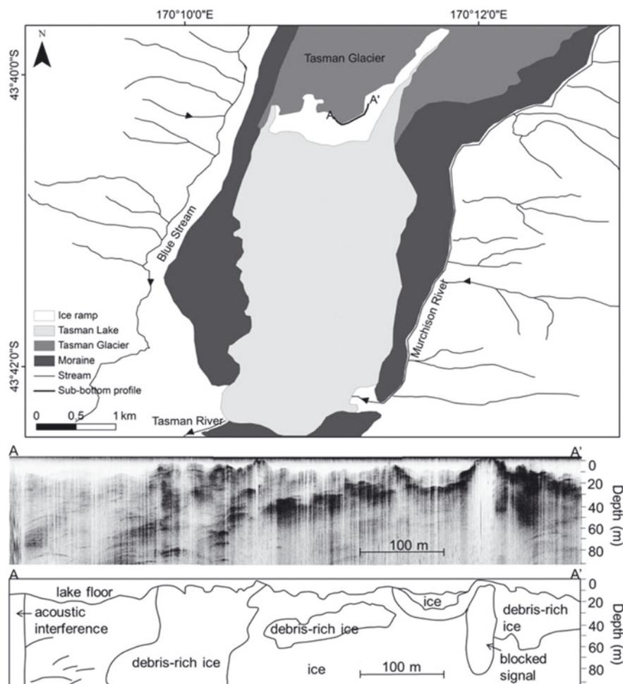
**Fig. 6.** Subaqueous terminus morphology of Tasman Lake in 2008. Line A–A' shows the location of the sub-bottom profile image. See Dykes and others (2011) for detailed bathymetry data collected at the same time as the sub-bottom profile data contained here.
