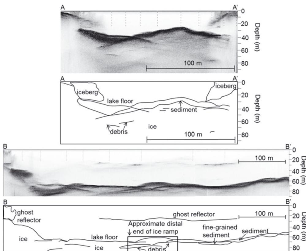
**Fig. 4.** Sub-bottom profile images and interpretation from Mueller Lake in April 2010. Profile locations are shown in Figure 3. The box shows the approximate distal end of the ice ramp.
