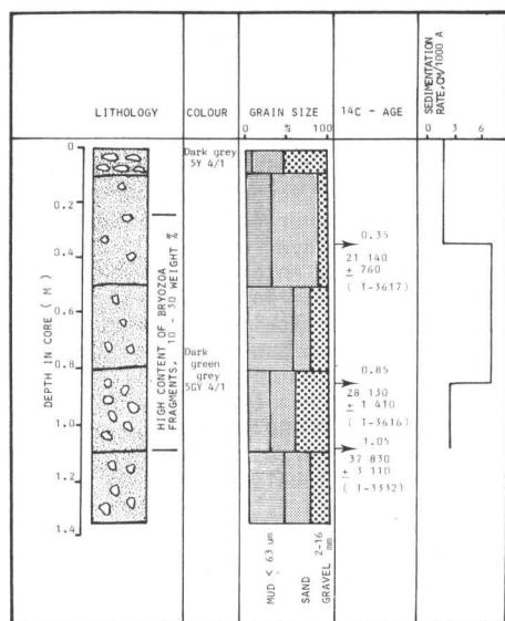
Fig.4. Characteristic lithological section of a core from the shelf break/upper slope outside Dronning Maud Land. X-ray analyses did not show any sign of lamination. Position: 72°19' S, 16°11' W, water depth 650 m.
