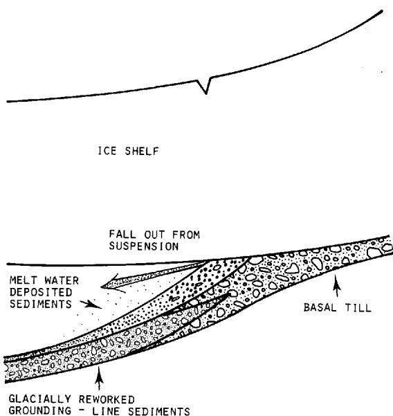
Fig. 5. A concept of the sediment distribution at the grounding line with outflowing melt water. Advance of the grounding line leads to glacial reworking of the melt-water deposits with mixing-in of basal till sediments.
