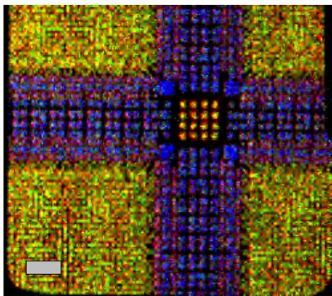
**Figure 2:** The X-ray image of a section of an IBM circuit board has dimensions of 1.2 cm x 1.2 cm, and it was acquired in 600 s. Yet this image was produced with the pnCCD without moving the stage, fully resolving spatial features, such as the wires in the center, which are approximately 150  $\mu\text{m}$  in diameter. Here the Cu X-rays are colored in red, the Au X-rays are in blue and the Ni X-rays are in green. The scale bar represents 1.4 mm on the image.
