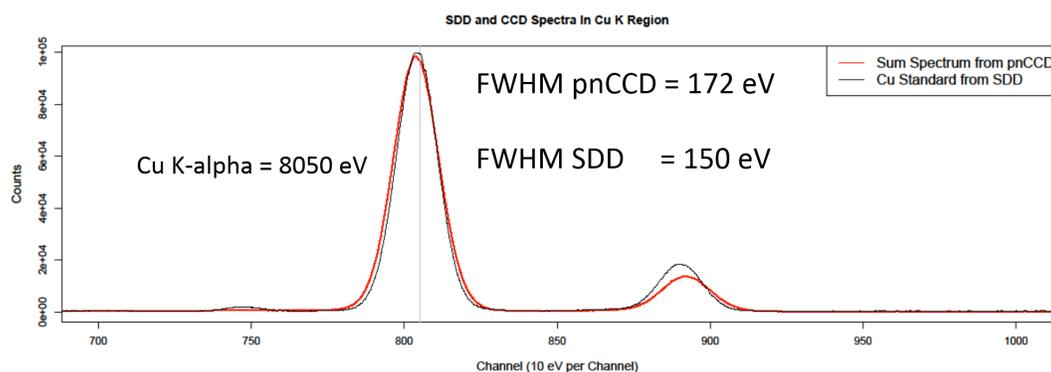
**Figure 1:** Spectral comparison of a spectrum from an SDD (black line) and a spectrum made with a pnCCD (red line). The pnCCD spectrum has an equivalent resolution of 152 eV at Mn K-alpha. The performance of the spectrometer at a count rate of over 200 000 counts/s is very good for imaging purposes.
