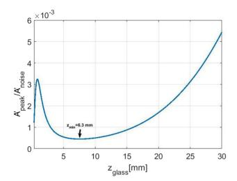
**Figure 8.** Beam area peak-to-noise ratio  $A'_{\rm peak}/A'_{\rm noise}$  at  $l=z_{w_{0,\rm NL}}$ , where the minimum ratio is obtained at  $z_{\rm glass}=6.3$  mm.
