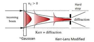
**Figure 1.** An Illustration showing the spatial shaping of a Gaussian beam affected by the temporal intensity change, which in turn modifies the medium.
