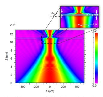
**Figure 16.** Beam propagation simulation showing spatial pulse variations. Starting from the bottom: beam convergence is observed after leaving the linear lens. A 'linear' waist is seen where the narrowest diameter is obtained (approximately the upper two-thirds of the figure). The nonlinear dielectric is represented by a cyan line. Major convergence occurs after leaving the nonlinear sample in air. The nonlinear waist is seen as the narrowest beam near the end (top).
