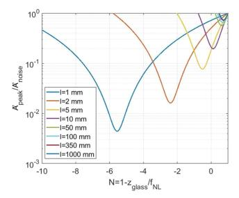
**Figure 4.** Peak-to-noise beam area ratios under various iris-to-glass distances (l) versus N values of  $z_{\rm glass}$  and C, which were set to 6.3 and 10.7 mm, respectively.
