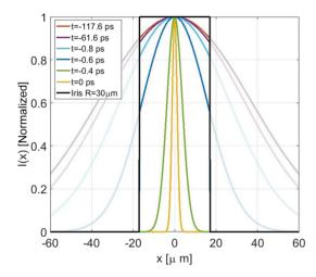
**Figure 11.** Spatial Gaussian pulses after experiencing the NL lens projected at the iris plane. The colored curves represent spatial pulses at various times. The (numerical) iris is represented by the black curve.
