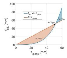
**Figure 7.** Kerr focal length as a function of glass distance from the beam waist position (blue), crossed with the linear  $f=z_{\rm glass}$  plot (orange). The intersection point of the two plots represents the precisely collimated case.
