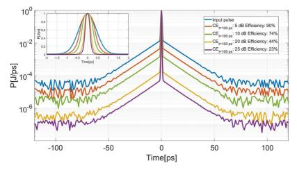
Figure 12. Contrast traces before (blue) and after the KL effect and hard aperture filter, for 70 (orange), 34 (green), 10.6 (yellow) and 4.8  $\mu$ m (purple) aperture diameters, applied upon the numeric Gaussian input beam. Inset: same plots in the time scale of a few ps surrounding the peak, provided for a more detailed observation.
