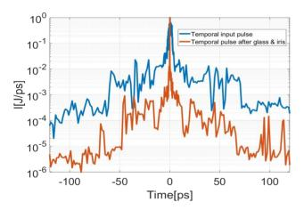
**Figure 13.** Measured pulse contrast before (blue) and after the KL effect and the clipping aperture (orange).
