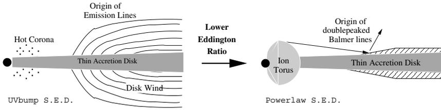
**Figure 3.** A sketch of how the structure of the accretion disk and its associated wind change as the Eddington ratio goes from high values ( $\dot{M}/\dot{M}_{\text{Edd}} \gtrsim 0.1$ ) to low values ( $\dot{M}/\dot{M}_{\text{Edd}} \lesssim 10^{-3}$ ). In the latter case the wind still exists but it is rather thin and inhomogeneous.
