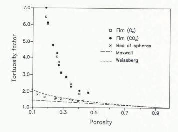
Fig.5. Tortuosity factor  $(D_0/D_m)$  versus porosity. The results obtained from firn samples are compared with values measured on a bed of spheres and theoretical curves. The lower curve is a theoretical lower bound for any isotropic porous medium and is derived from a formula by J.C. Maxwell describing the electrical conductivity of inhomogeneous substances; the upper curve is a theoretical lower bound for a porous medium consisting of overlapping spheres (Weissberg 1963).
