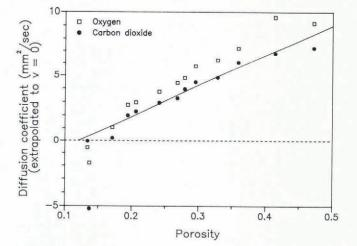
Fig.4. Extrapolated molecular diffusion coefficients measured on firn samples from Siple Station (Antarctica), versus the firn porosity. The line is a linear regression through the values for  $CO_2$ .
