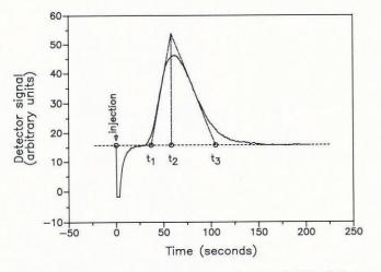
Fig.2. Typical elution peak of a  $\delta$  input of CO<sub>2</sub> fed to the carrier gas after passing through the firn sample.
