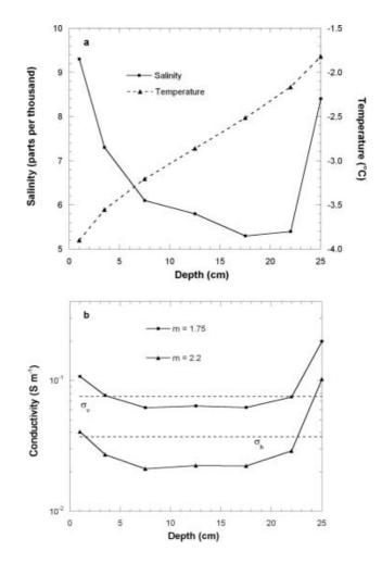
**Fig. 6.** (a) Salinity and temperature profiles measured on a sea-ice core from site 2 (Table 1). (b) Bulk sea-ice conductivity computed from the data in (a) using Archie's law, for different values of the exponent *m*. The horizontal dashed lines denote the horizontal ( $\sigma_h$ ) and vertical ( $\sigma_v$ ) conductivities determined from interpretation of the in situ d.c. geoelectrical sounding data.
