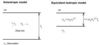
**Fig. 3.** Equivalent transversely isotropic (left) and isotropic (right) 1-D d.c. geoelectrical models. For the anisotropic case,  $\sigma_v$  and  $\sigma_h$  are the conductivities in the vertical and horizontal directions respectively, and  $t_a$  is the layer thickness. In the isotropic model,  $\sigma_m$  and t are the equivalent upper-layer conductivity and thickness respectively. In both models, the conductivity of the bottom layer (sea water) is isotropic.
