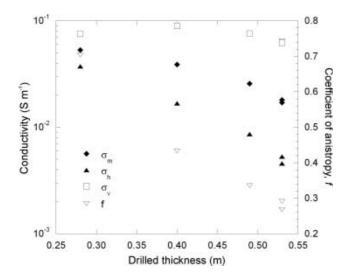
**Fig. 4.** Graph of in situ sea-ice conductivity and coefficient of anisotropy vs drilled thickness for five d.c. geoelectrical soundings on level sea ice in East Antarctica.  $\sigma_h$  and  $\sigma_v$  are the interpreted sea-ice conductivities in the horizontal and vertical directions respectively.  $\sigma_m$  is the conductivity of the equivalent isotropically conductive layer and is equal to the geometric mean of the horizontal and vertical conductivities.
