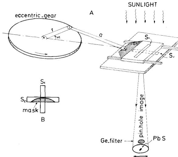
Fig. 2. Schematic drawing of the device used for the IR intensity measurements (dimensions are quite arbitrary); for the explanation see text.
