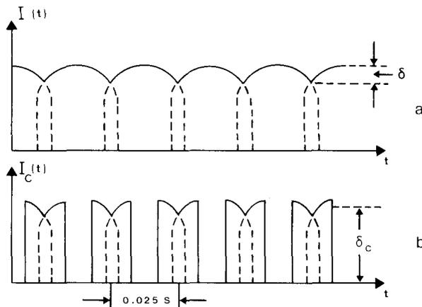
Fig. 3. Schematic plots of the PbS output for the recording of the differential intensity signal (a) and the calibration (b). Frequency of modulation is 40 Hz.
