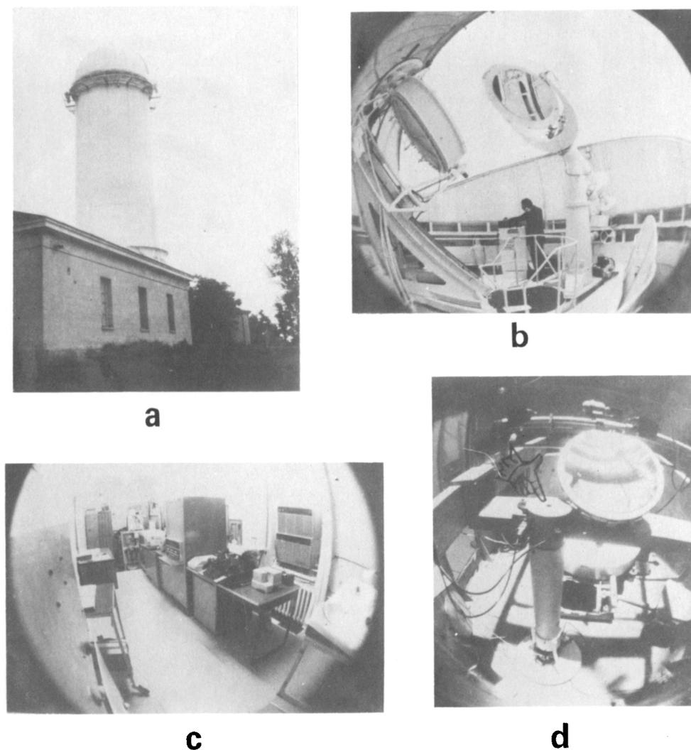
Fig. 1. General view of the Crimean Solar Tower Telescope and the instrumentation. (a) Solar Tower; (b) coelostat mirrors (about 24 m above the ground level); (c) the solar magnetograph (used also for Doppler velocity measurements and, partially, for the recording of IR observations) and the computer; (d) the diagonal flat mirror used for the Doppler velocity measurements and the IR device (its entrance aperture is indicated) illuminated by a parallel beam.
