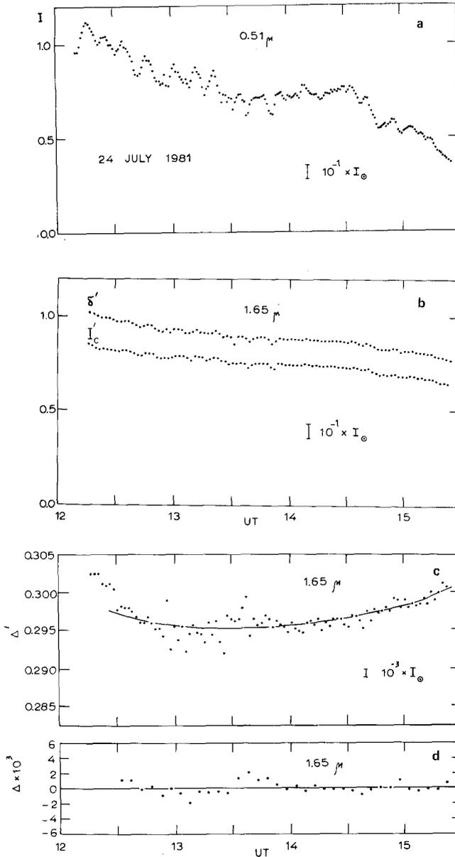
Fig. 5. An example of intensity records obtained on 24 July 1981 under poor atmospheric conditions (hazy sky): (a) the run of solar intensity measured at  $\lambda 0.51 \mu\text{m}$ ; (b) the same for  $\lambda 1.65 \mu\text{m}$  (for the two IR signals,  $\delta'$  and  $I_c''$ ); (c) the ratio of two IR signals,  $\Delta' = \delta' / I_c''$ ; (d) the plot of residuals  $\Delta = \Delta' - \Delta_0$  (5-min averages).
