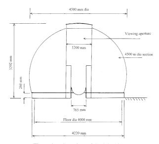
Figure 1—Dimensions of the 4.5 m dome.
