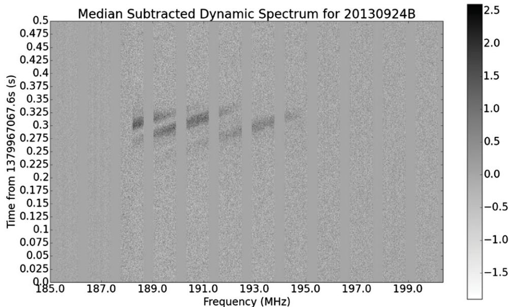
**Figure 6.** A dynamic spectrum from MJD 56559 spanning 0.5 s and showing short lived multi-path interference fringes from TV Channel 8 (8 MHz centred approximately around 191.5 MHz). The median from each frequency bin was subtracted before plotting. Time is averaged to 1 ms (the plot spans 0.5 s) and frequency is kept at 10 kHz. Once again, the vertical lines between coarse channels are visible through the variable emission.
