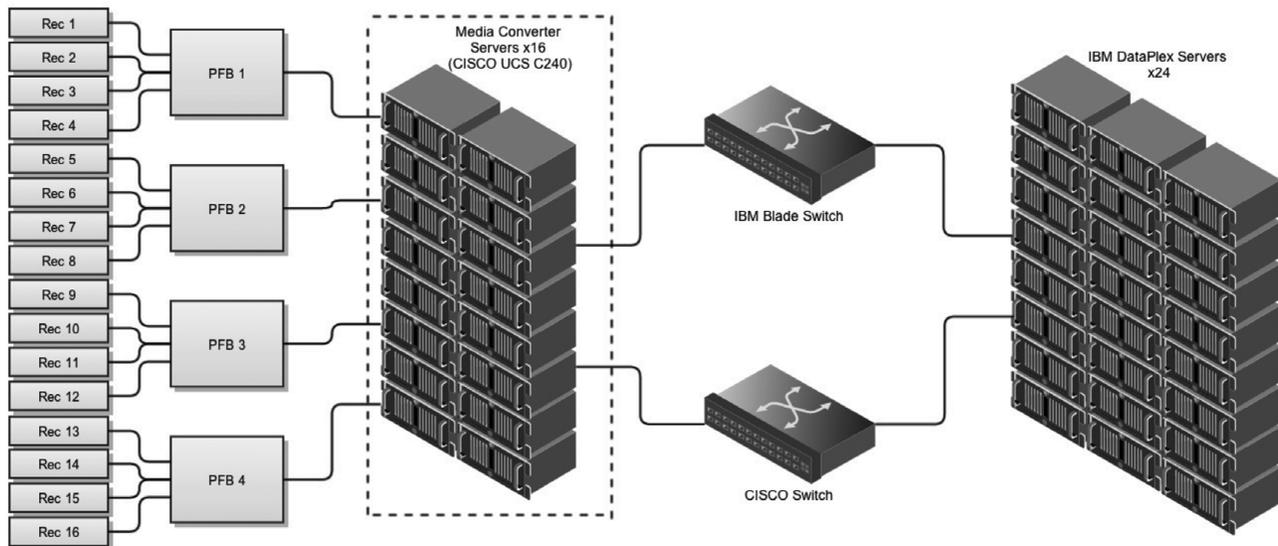
**Figure 1.** Simplified illustration of the MWA digital signal path. For the VCS mode, the baseband data between the fine channel polyphase filter bank (PFB) and the X-engine of the correlator are written to local RAID's on the 16 media converter servers (highlighted with a dashed box). This gives us  $100 \mu\text{s}$  resolution and frequency channels 10 kHz wide.
