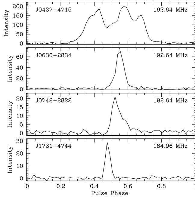
**Figure 2.** Pulse profiles of four different pulsars observed with the VCS mode covering a range of DMs and periods (see Table 1 for values) to demonstrate the flexibility of the instrument. There are 64 bins, spanning the pulse period for each pulsar.
