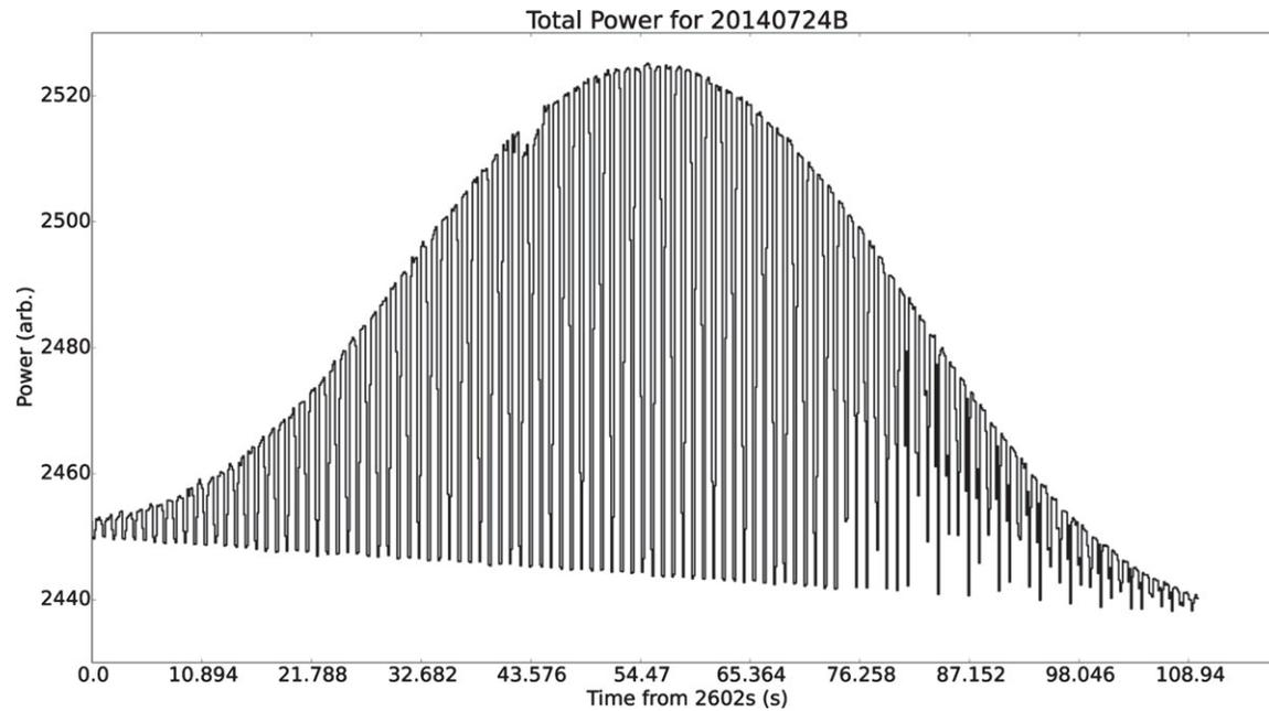
**Figure 5.** Total power (summed over tiles and frequencies) plot showing the effect an Orbcomm satellite has on a 184.96 MHz observation when transmitting within our beam, the envelope of the signal amplitude tracing out the tile gain pattern. These data have been averaged to 130 ms. Note the 1 Hz power variations, which would cause problems for blind periodic pulsar searches. Reference time on axis is seconds from the beginning of the observation.
