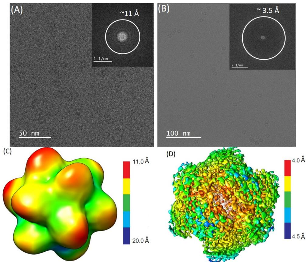
**Figure 1.** CryoTEM image in (A) is acquired with OneView and while the image in (B) is acquired with K2. Rings in the inserted FFTs represent their resolution. Resolution maps of 3,4-PCD proteins shown in (C) and (D) are generated from the processed OneView and K2 datasets.
