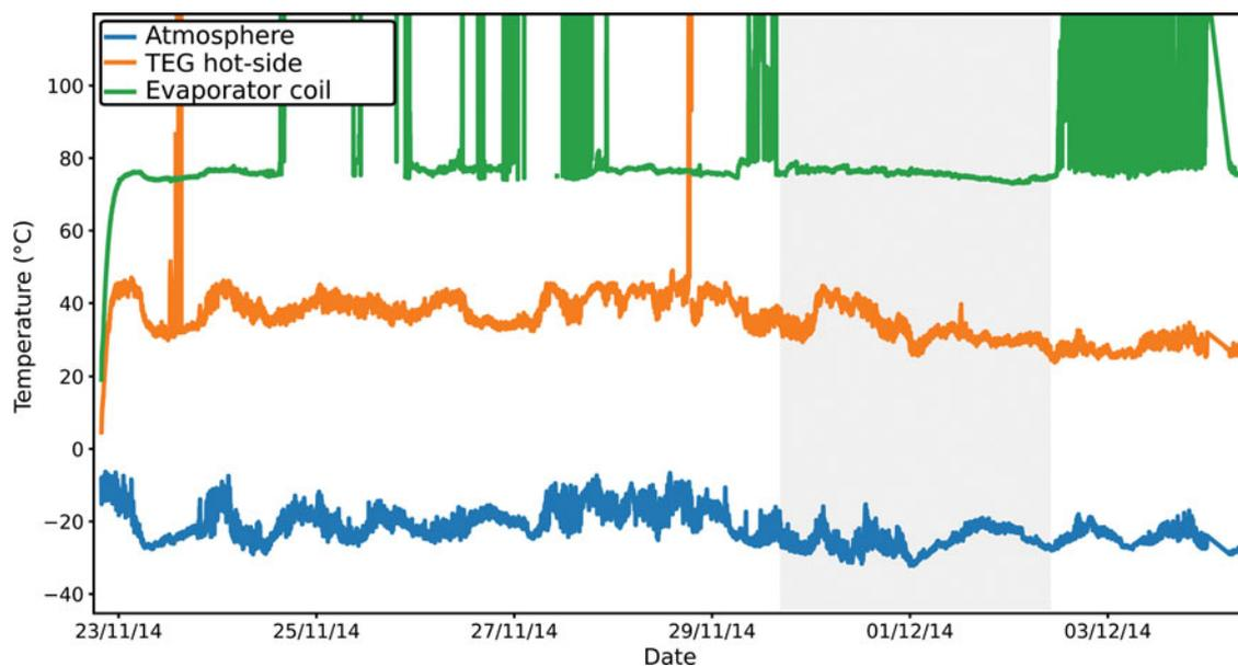
**Fig. 5.** Seebeck generator temperature data from the ~11 days of deployment showing the temperature of the evaporator coil (top), the hot side of the thermoelectric generator (TEG) chip (middle) and the atmospheric temperature (bottom). The anomalous data in the TEG hot-side and evaporator coil series are thought to be caused by a poor electrical connection to the data logger. The shaded region denotes the time period plotted in the scatter plots in Fig. 6.
