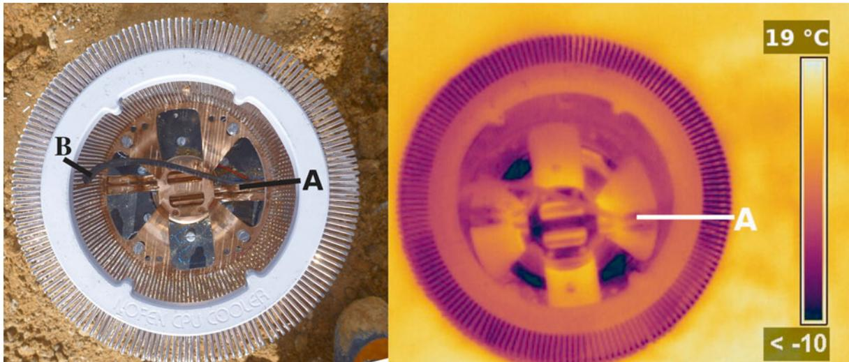
**Fig. 8.** Top view of the Seebeck generator (left) and corresponding image in thermal infrared (right). The heat pipes incorporated into the heat sink assembly (marked A) appear cold, suggesting that they were not operating correctly (note that these heat pipes are distinct from that labelled B in Fig. 1). The atmospheric temperature sensor is marked B.
