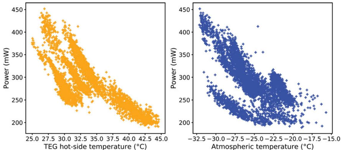
**Fig. 6.** Scatter plots of thermoelectric generator (TEG) hot-side temperatures (left) and atmospheric temperatures (right) against power output for the time period denoted by the shaded region in Fig. 5. Each data point represents a 1 min average of the recorded values.
