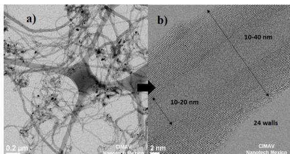
**Figure 1.** a) TEM and b) HRTEM images of multiwalled carbon nanotubes.
