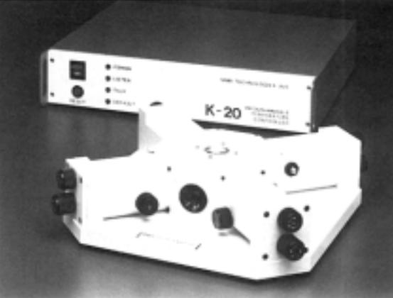
**MMR's Variable Temperature Micro Probe System** (one to seven probes) is designed to provide controlled cycling of sample temperature from 80K to 730K (450°C).
