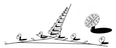
**Figure 3.2** First revision of the original MMA concept with the 6 m diameter antennas in a Y-configuration on tracks and the 3 m diameter antennas mounted on a steerable platform. Credit: NRAO/AUI/NSF, CC BY 3.0.
