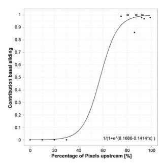
**Fig. 3.** Empirical function to estimate the contribution of basal sliding to the glacier surface velocity (z) based on the ratio of the total glacier area and the glacier area upstream of a particular location assuming no sliding in the upper parts.
