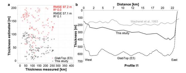
Fig. 6. (a) Koxkar GPR ice thickness measurements vs. thickness estimates based on Eqn (4) (This study) and Eqn (3) (GlabTop). (b) Longitudinal profile along South Inylchek Glacier (Profile I1, Fig. 4b) showing thickness measurements from Macheret and others (1993) and thickness estimates from this study.
