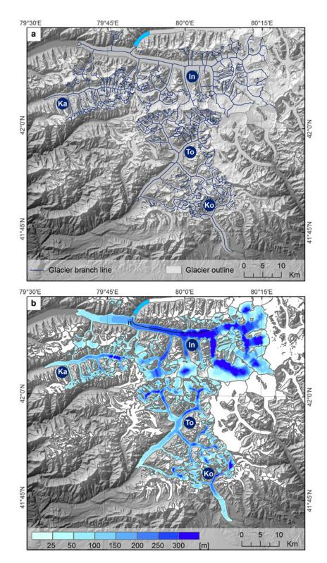
Fig. 4. (a) Glacier branch lines for Koxkar, Tomur, Kaindy and South Inylchek glaciers, (b) Glacier ice thickness for South Inylchek, Kaindy, Tomur and Koxkar glaciers. I1 indicates the position of the longitudinal profile measured by Macheret and others (1993).
