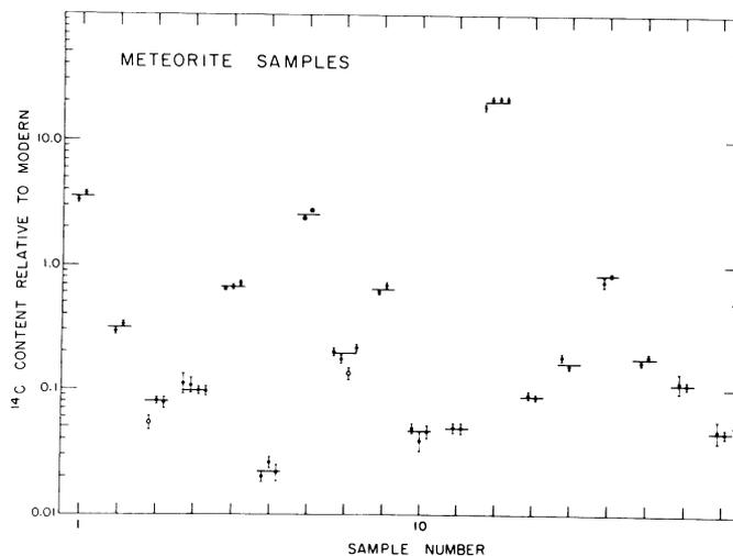
Figure 3.  $^{14}\text{C}$  content of meteorite samples. Error bars are counting statistics only. Open points not included in mean values shown by horizontal bars.
