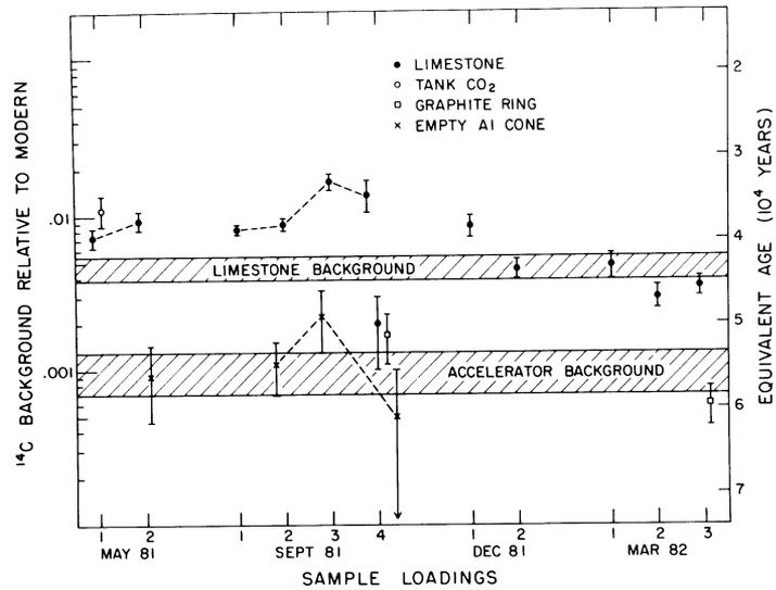
Figure 1.  $^{14}\text{C}$  background in the Chalk River MP Tandem Accelerator, 1981-82
