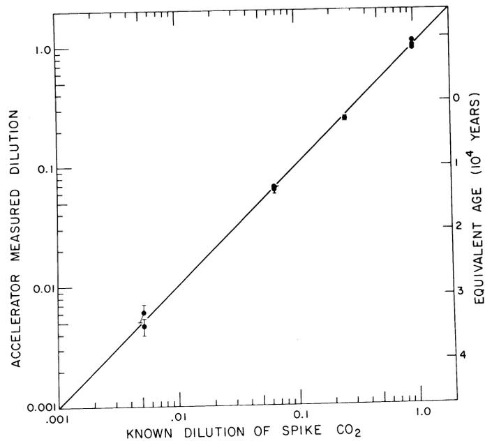
Figure 2. Accelerator measurements of quantitatively diluted spike  $^{14}\text{CO}_2$
