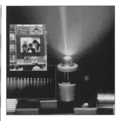
**ON THE COVER:** Blue GaN-based laser diode operated at room temperature under pulsed conditions. TOP INSET: Outdoor display in downtown Tokyo, utilizing GaN light-emitting diodes. BOTTOM INSET: GaN-based light-emitting diodes of different InGaN composition, leading to colors from blue to yellow. For more information, see the section that begins on page 17.
