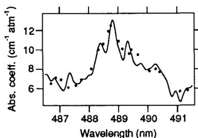
Figure 2. Comparison of our measured NO<sub>2</sub> absorption coefficient (solid line) and that published by Woods and Jolliffe (1978) (points).
