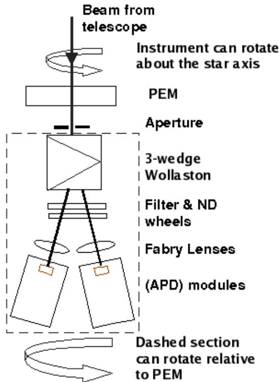
**Figure 1.** Schematic of PlanetPol. There are two identical channels with only one shown: the object channel is on the telescope axis and the sky channel is offset by 95mm. The instrument is rotated through 45° to measure the second linear Stokes parameter. The analyser, together with the filter and detector assemblies, is rotated by 90° (from -45° to +45° relative to the PEM axis) changing the polarity of the modulated signal thereby minimizing systematic errors.
