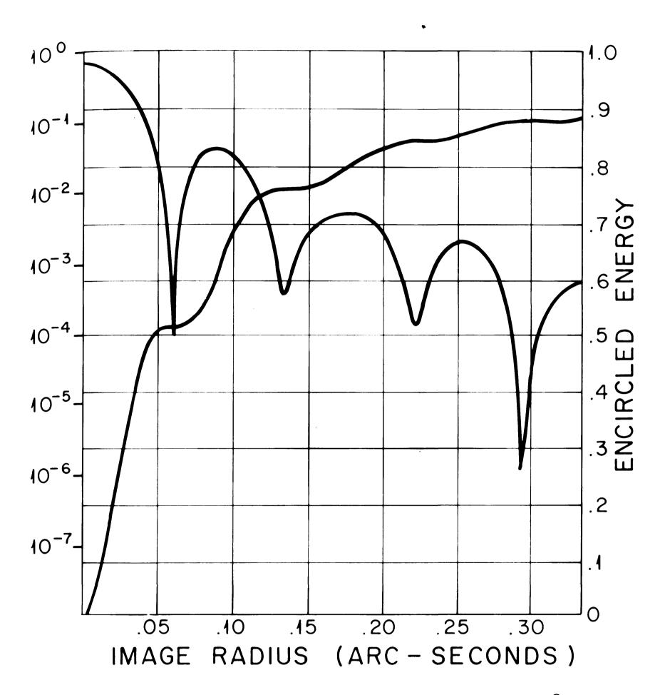
Figure 2: The expected optical performance ( $\lambda6328\mbox{\ensuremath{\mbox{A}}}$ ) is illustrated in terms of the image surface brightness distribution and the encircled energy. The central obscuration and deviations from perfect mirror figure and alignment have been incorporated in these predictions.
